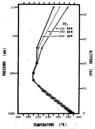
Fig. 16. Vertical distributions of temperature in radiative convective equilibrium for various values of CO<sub>2</sub> content.
