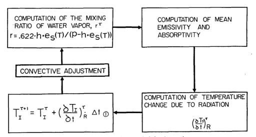
Fig. 2. Flow chart for the numerical time integration.
