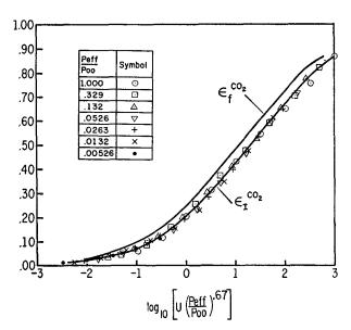
Fig. 28. Slab absorptivity  $\epsilon_I$  and column absorptivity  $\epsilon_I$  of CO<sub>2</sub> at 300K. Bandwidth is assumed to be 250 cm<sup>-1</sup>.
