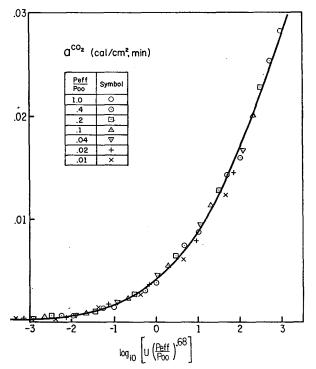
Fig. 25. The rate of absorption of solar radiation by CO<sub>2</sub>.
