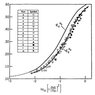
Fig. 30. Slab and column absorptivity of 9.6- $\mu$  band of O<sub>3</sub>. Run means the run of experiments by Walshaw (1957). Bandwidth is assumed to be 138 cm<sup>-1</sup>.
