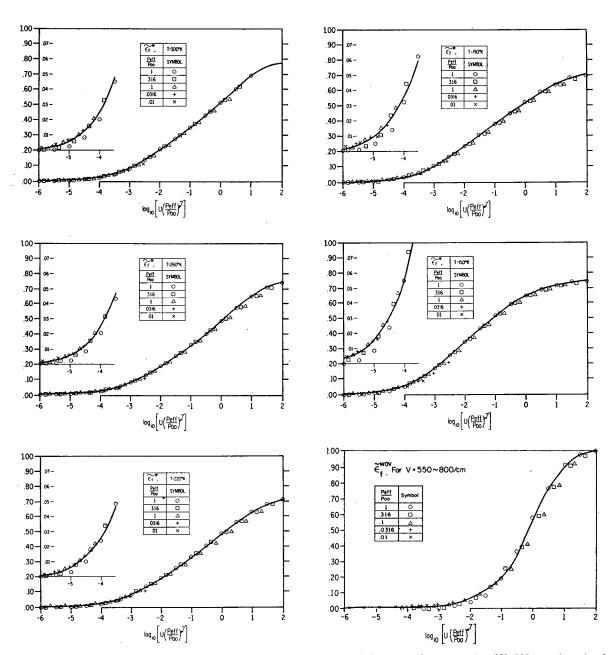
Fig. 26. The mean slab absorptivity of H<sub>2</sub>O, from which the contribution of the range of wave number 550-800 cm<sup>-1</sup> is omitted.
