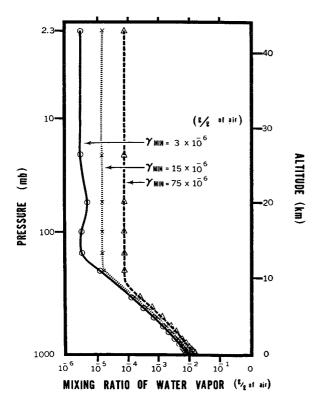
Fro. 13. Vertical distribution of water vapor mixing ratio corresponding to the equilibrium status shown in Fig. 12.
