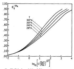
Fig. 29. Slab absorptivities of CO<sub>2</sub> at various temperatures.
