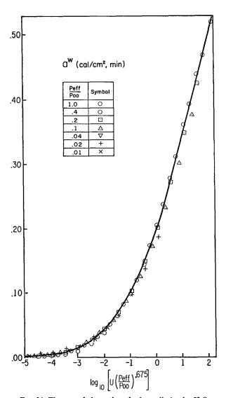
Fig. 24. The rate of absorption of solar radiation by  $H_2O$ .
