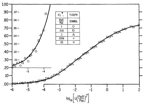
Fig. 27. Emissivity of H<sub>2</sub>O from which the contribution of the wave number range 550-800 cm<sup>-1</sup> is omitted.
